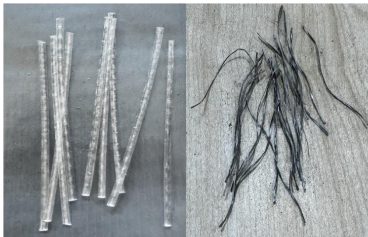
Visual 1. Image of Polypropylene Fibers (Type A on the Left, Type B on the Right)
