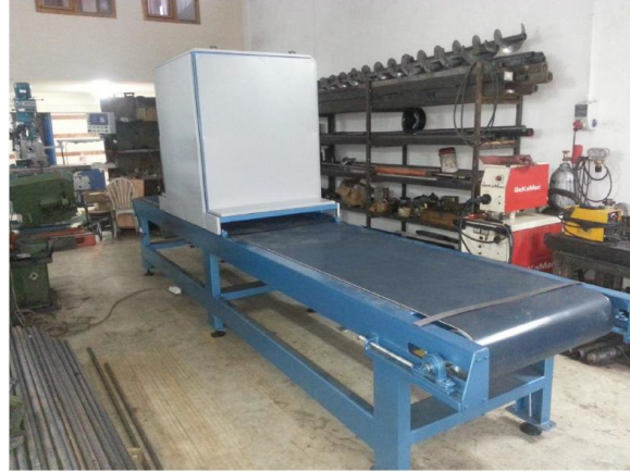
Figure 1. Machine vision system designed and manufactured as a result of the "Automatic Classification of Natural Stone Plate with Machine Vision" project numbered 1120167 and the doctoral thesis of the same name [1]
