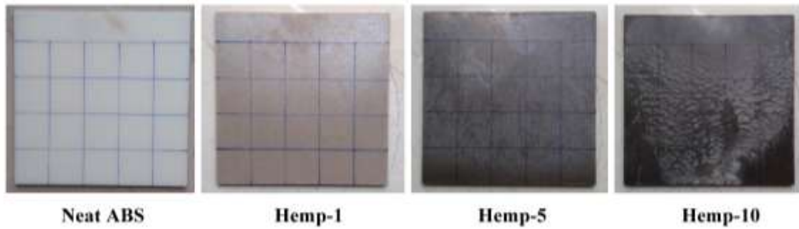
Figure 2. Determined hammer hit points on plate specimens
