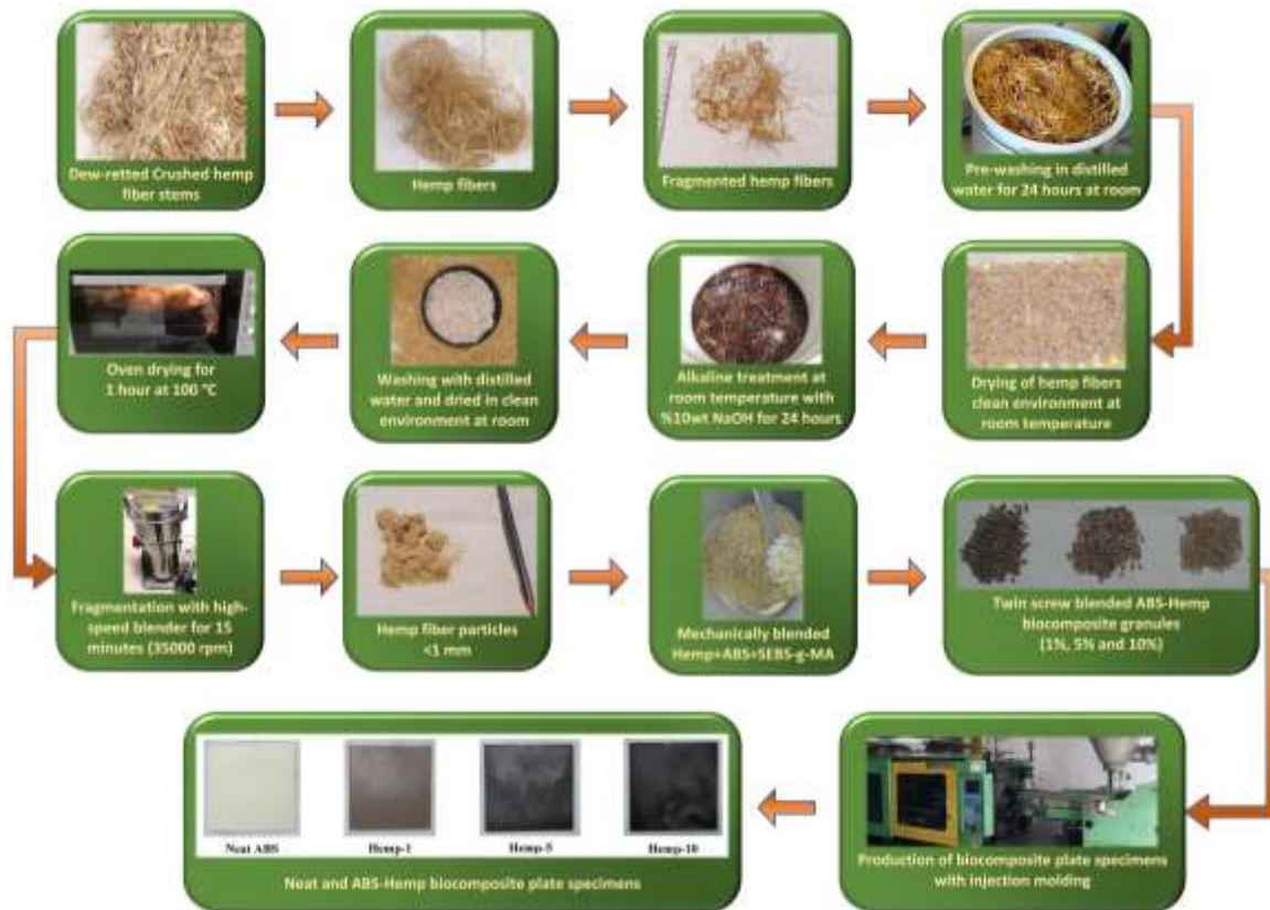
Figure 1. Production process of ABS/Hemp biocomposite plate specimens.
